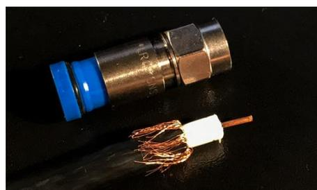
Fitting connector – How braid should be trailed/trimmed.
