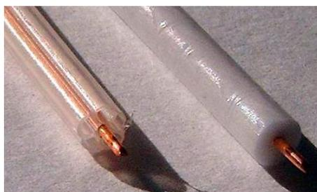
Bad-CT100 (Air Spaced) vs. Good-WF100 (Foam Fill)
