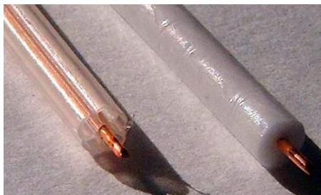
Bad-CT100 (Air Spaced) vs. Good-WF100 (Foam Fill)
