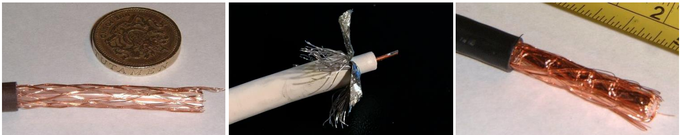
Bad – Low loss TV coax cable, insufficient shielding
