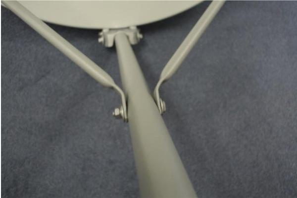
This closer view shows the smaller arms connected to the main arm
